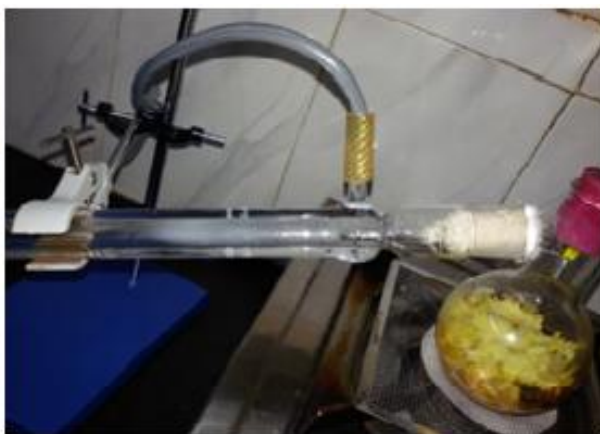
Condensation of Arka vapours
