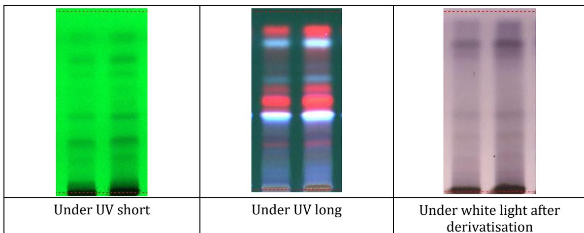
**Figure 7: HPTLC plate visualized under UV short, UV long and white light**
