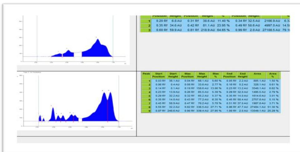
Figure 8: Graphical representation of Track 1 and 2 in HPTLC
