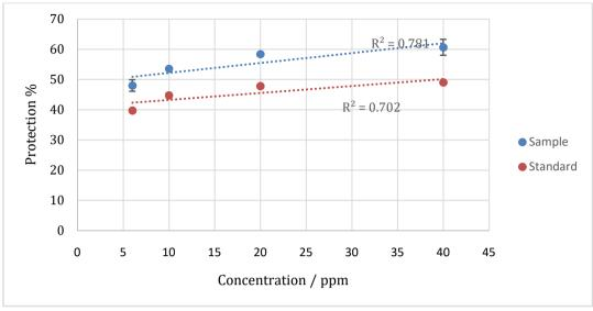
Figure 4: Percentage protection vs concentration of ALEPA and asprin standard
