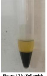
Figure 12 b: Yellowish supernatant after centrifugation at 300 rpm for 20 min
